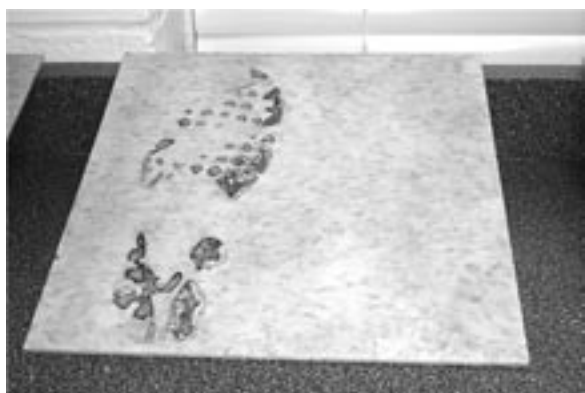
Figure 3. A shoe print developed on vinyl tile using the amido black method for visualizing bloody shoe prints
