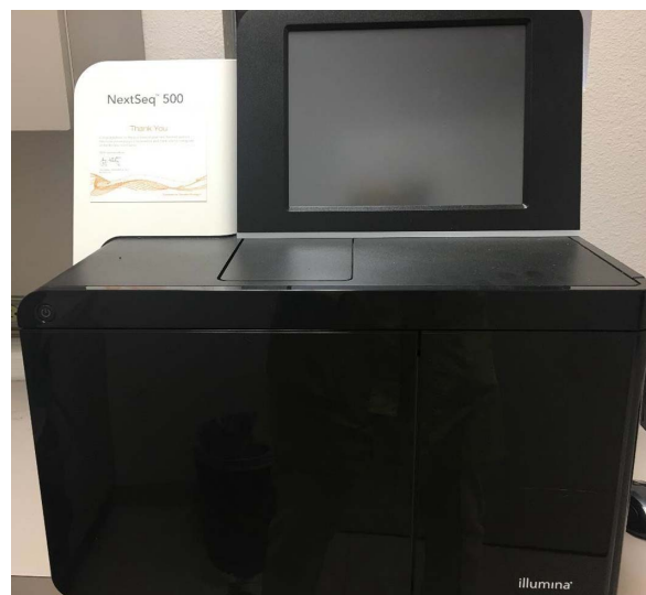
Figure 1. NextGen Sequencing. Next-generation sequencing (NGS) is a powerful platform that enables the sequencing of millions of DNA molecules from multiple patients simultaneously.
